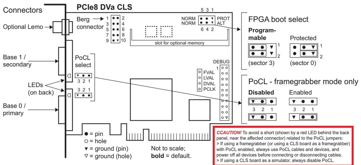
**Figure 2. Legacy (“DV”) products: PCI DV CLS and PCIe8 DV CLS**
