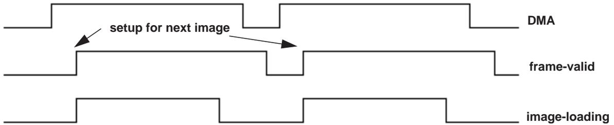
DMA starts with the program's call to `edt_start_buffers(pdv_p, 1)`. After the CLS has 16 KB of data, it starts sending data to the frame grabber. At the same time it sends the FVAL interrupt to the driver, which in turn calls `setup_clsim_event`. Immediately after the program calls `edt_start_buffers`, it loads the next image into the buffer most recently sent (so the buffer being loaded is just behind the buffer being sent).
