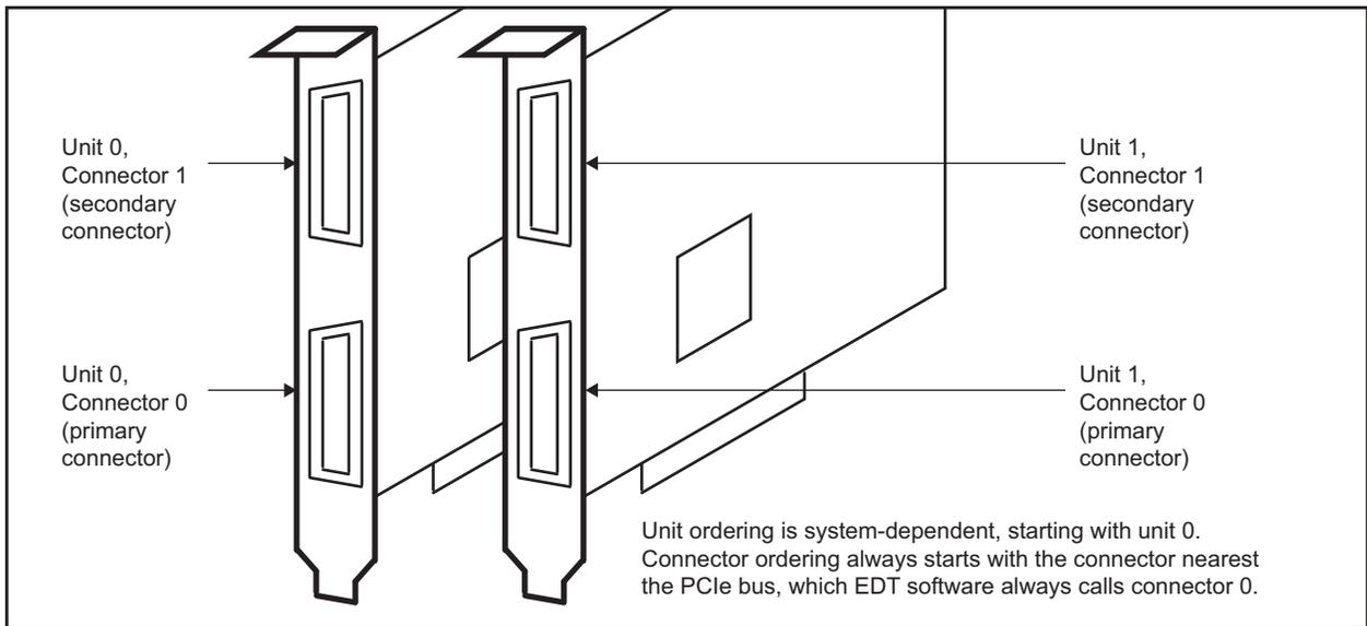
If you are using multiple EDT boards (units), or multiple connectors on a single EDT board, the software provides a unique handle to represent each unit and connector. Unless you specify something else, any application (either your own or EDT's) seeking access to the devices will default to unit 0, connector 0.
