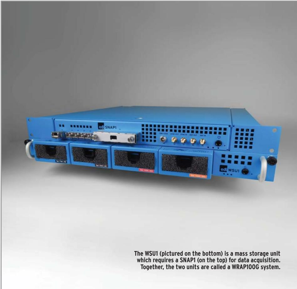
The WSU1 (pictured on the bottom) is a mass storage unit which requires a SNAP1 (on the top) for data acquisition. Together, the two units are called a WRAP100G system.
