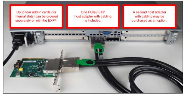
Figure 1. Expansion case (rear view) with included power cable, PCle host adapter, and PCle cable
