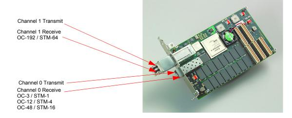
Figure 1. Connector Pinout
