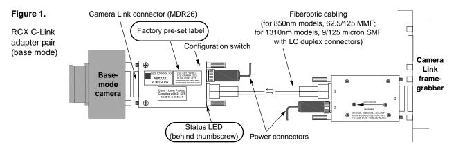
**First, verify presets.** On each adapter's factory preset label (circled in Figure 1), find "Blink Code *N-N.*" The first number tells you the device to which the adapter connects (1 for camera, 2 for framegrabber); the second number tells you the adapter's constraints for pixel clock rate and bit range, as shown below.
