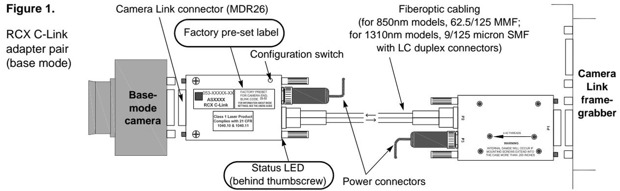
**First, verify presets.** On each adapter's factory preset label (circled in Figure 1), find "Blink Code N-N." The first number tells you the device to which the adapter connects (1 for camera, 2 for framegrabber); the second number tells you the adapter's constraints for pixel clock rate and bit range, as shown below.
