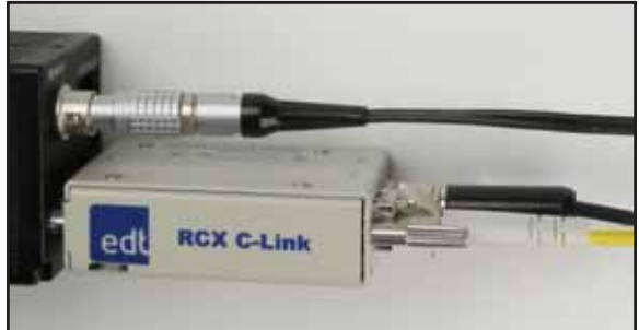
An extender connected to a camera
