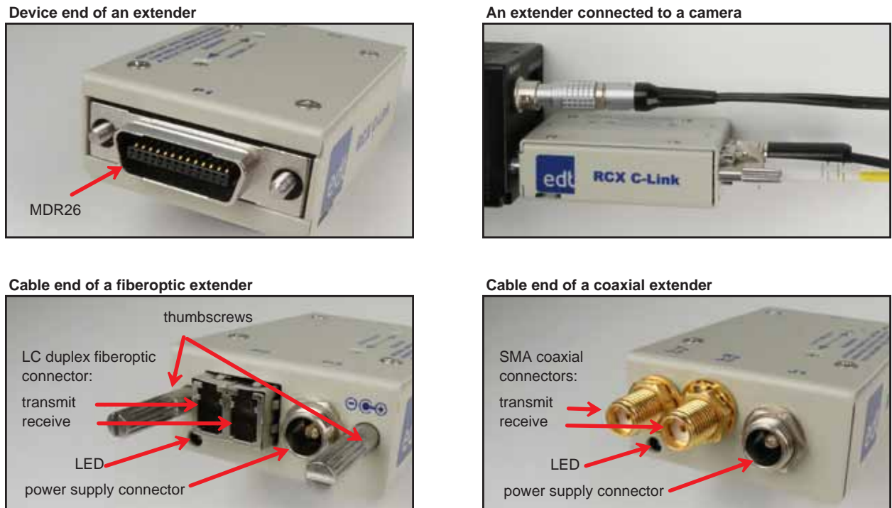
Figure 2. Connectors and features on EDT extenders
