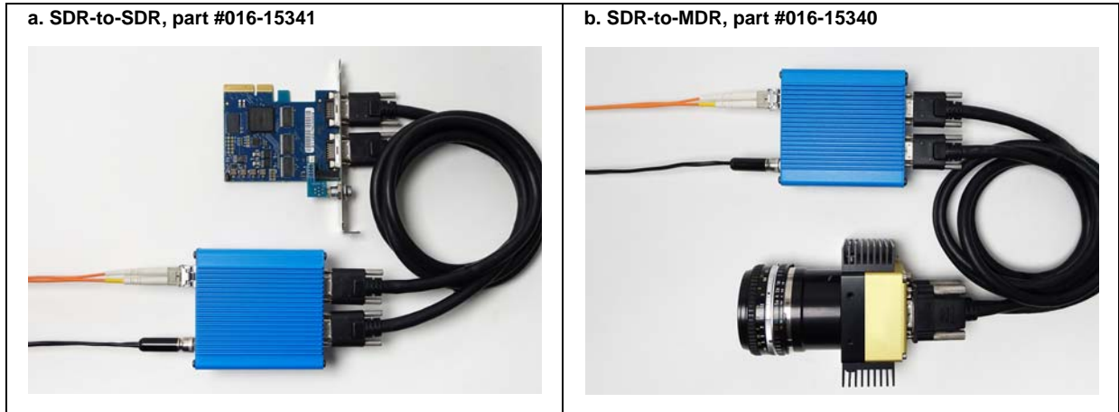
Figure 2. Connecting Camera Link cables to the VisionLink XF
